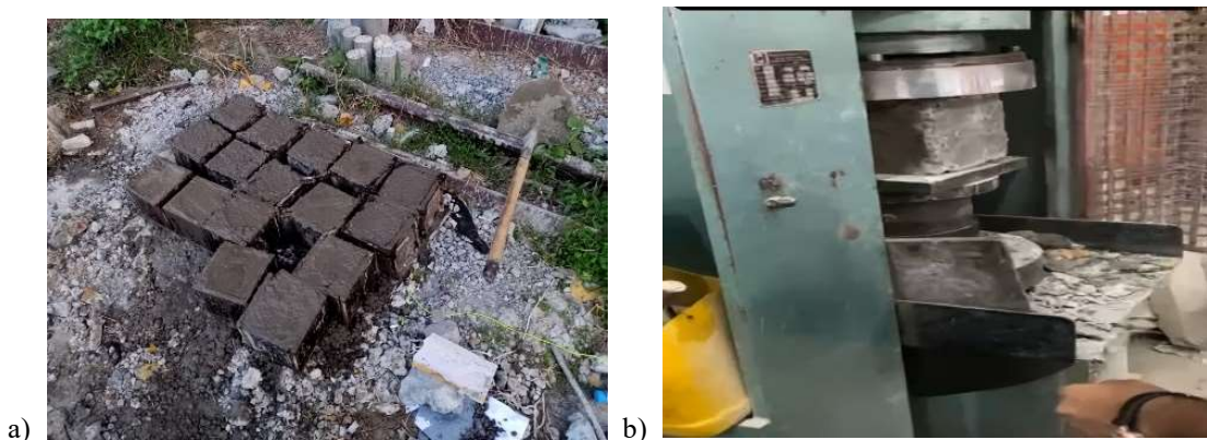
Figure 5: Cubes, a. casting of cubes, and b. testing of cube
